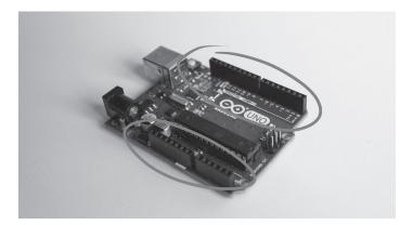
In this sketch, though, we won't be attaching any wires to anything—instead, we're going to work with the Arduino's **onboard LED**, which is an LED light that is hard-wired to pin 13 on the Arduino (it's labeled with an L on the surface of the Arduino board). Because it's already connected to pin 13, we won't need to add any extra electronics.
