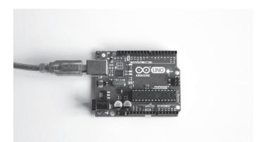
Now we have to make sure the computer knows what kind of Arduino board it's uploading to. Go to Tools > Board on the menu bar and select "Arduino Uno" from the rather lengthy list of possible boards.
